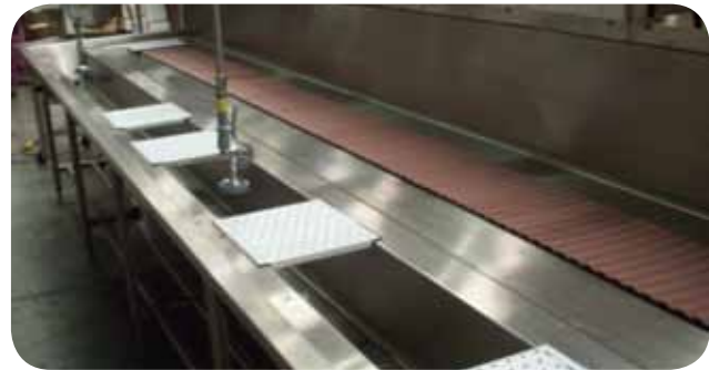
Trough bridges and obstruction-free pre-rinse sprays
